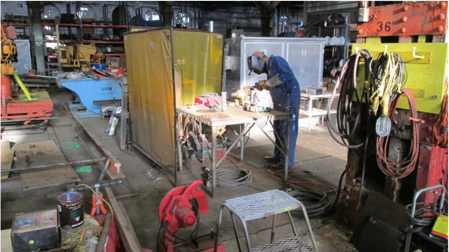
Cliff uses a grinder on the welds of the new step he just made for the other side of the Kalamazoo
