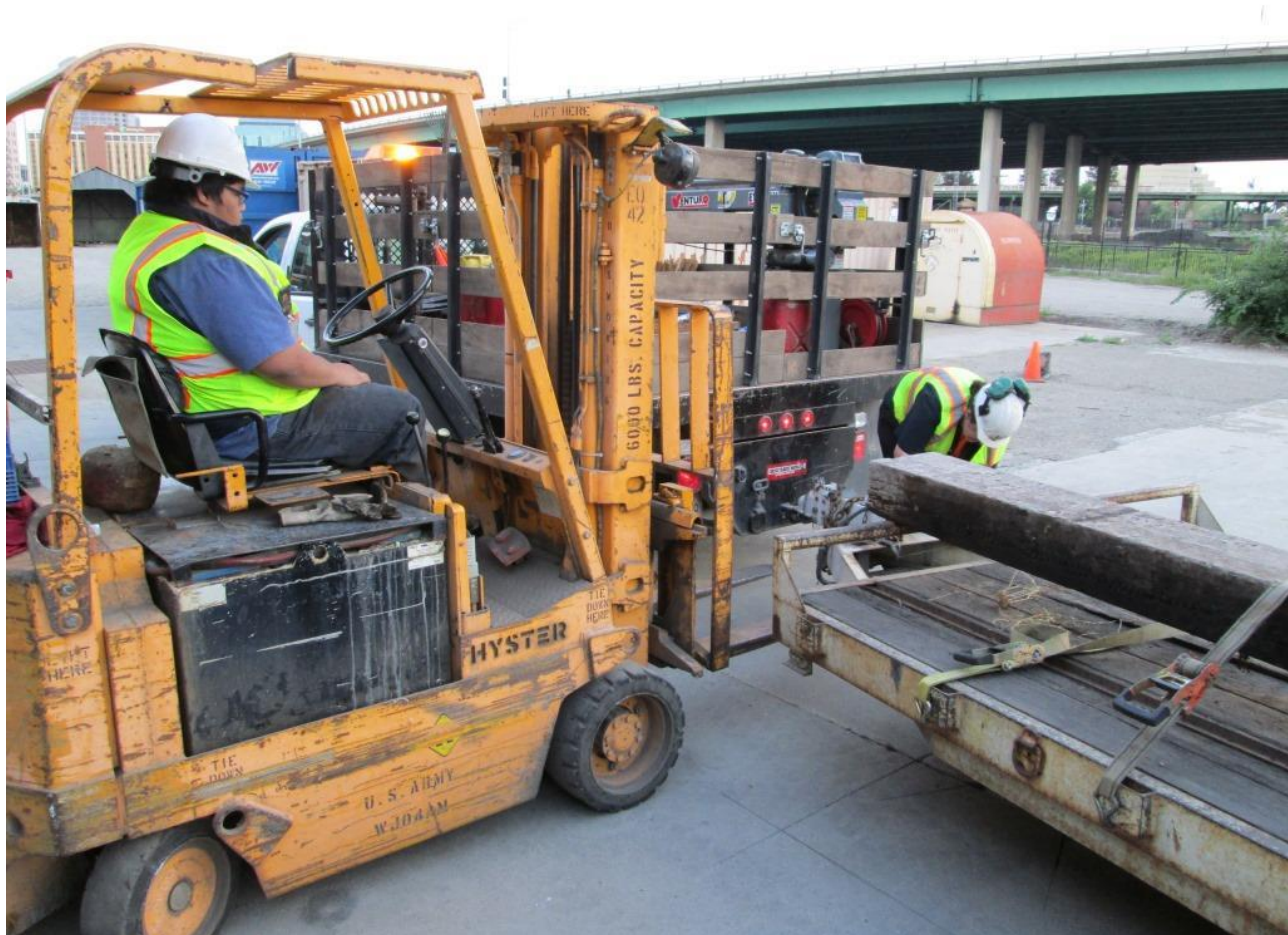
Anthony on the forklift gives the trailer a bit of a lift to relieve the presser on the hitch-latch so that Heather can remove it
