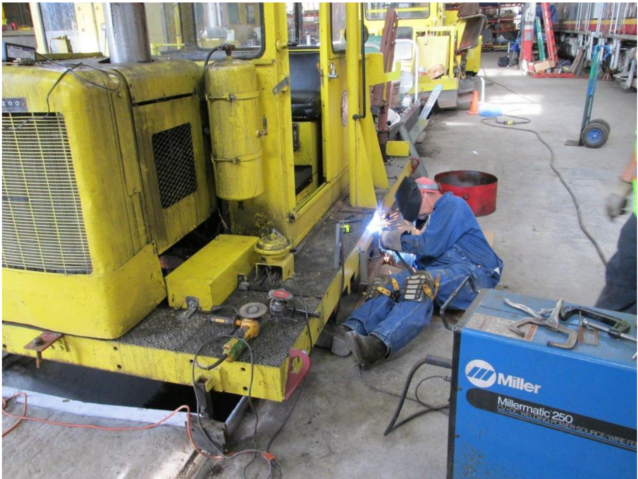
Cliff welds a new step onto the deck of the Kalamazoo
